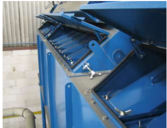
3 Convincing in practical application: modular design, easy accessibility and filter pack changeout from the clean air side
