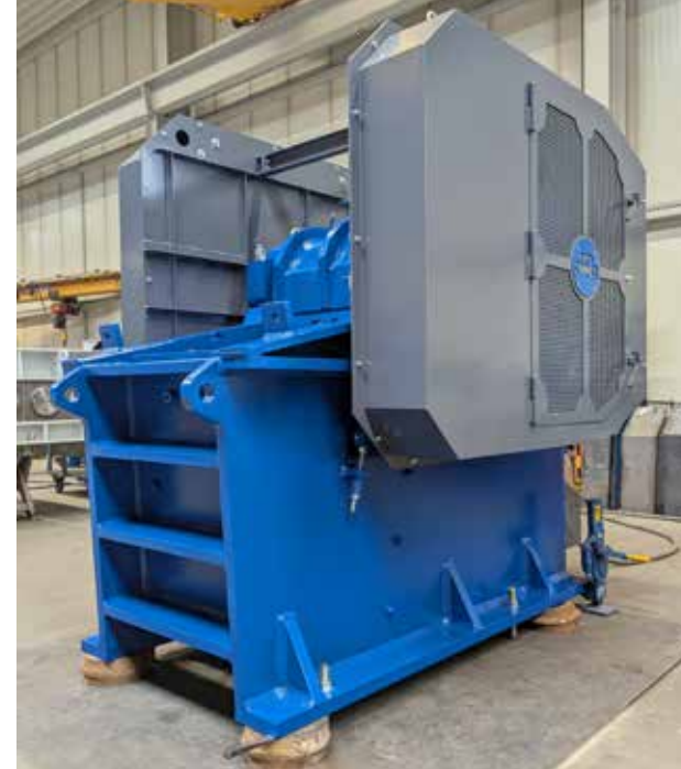
Robuster Backenbrecher Robust jaw crusher
