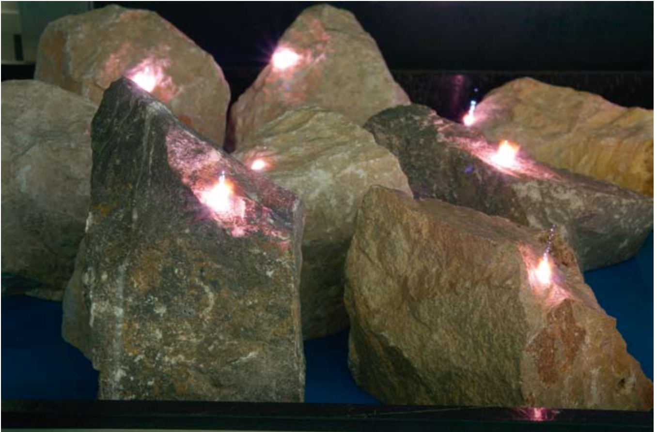
Laser-induced plasma on rock sample
