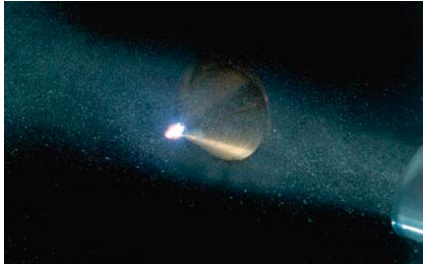
3 Image of a laser-induced plasma in an air current with a concentration of boring dust
