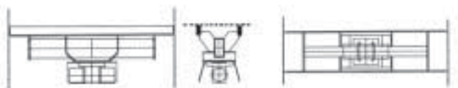
6 Diagram of a drive traverse excited by balancing weights of the screening machine, type Fine-Line, from HAVER & BOECKER
