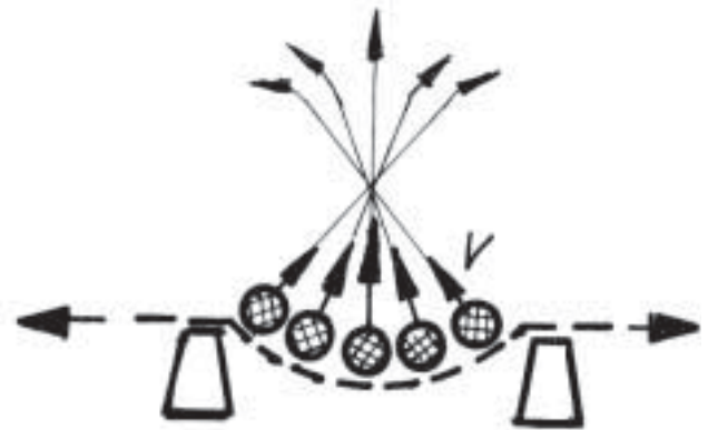
8 Schematic representation of the speed vectors v during particle motion on the flip-flop screen deck
