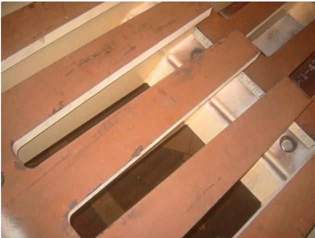
4 Steps of the grizzly made of Hardox 450 with 60 mm thickness
