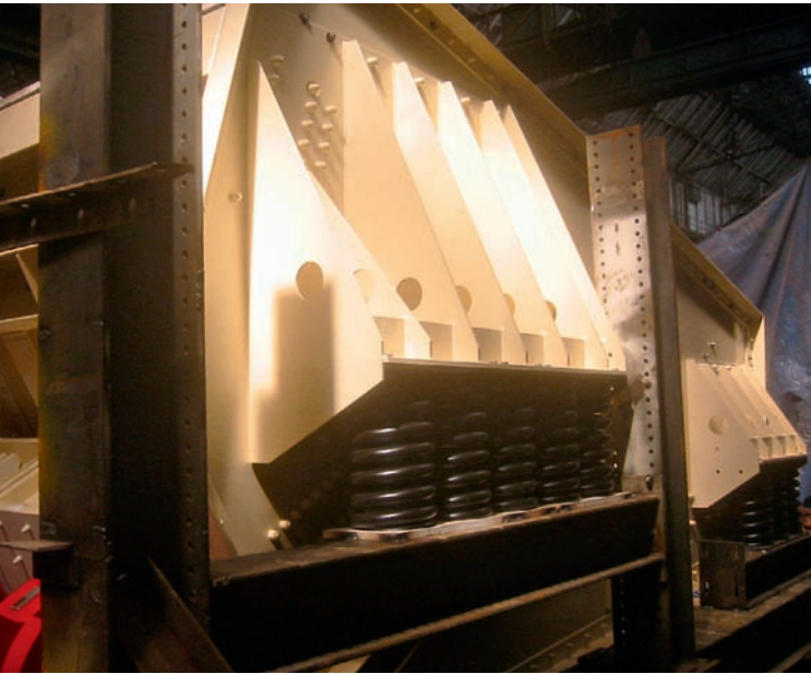
2 Support brackets for the springs of the coarse screen
