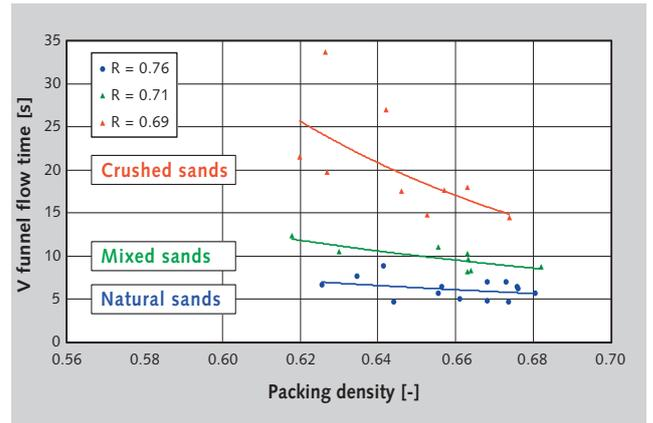
6 Relationship between the packing density and V funnel flow time at the same slump
