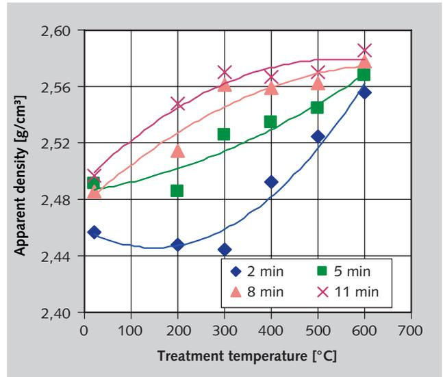
11 Starting material 4/8 – influences of the treatment temperature and the milling time on the apparent density of the coarse product
