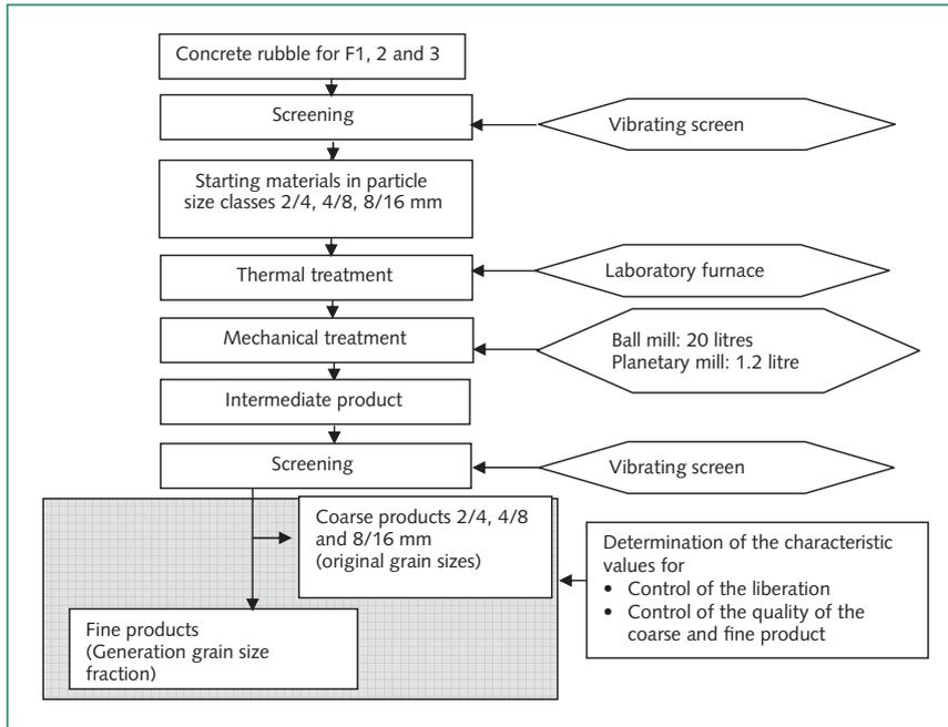
1 Flow sheet showing the test procedure (SP: Focus)
