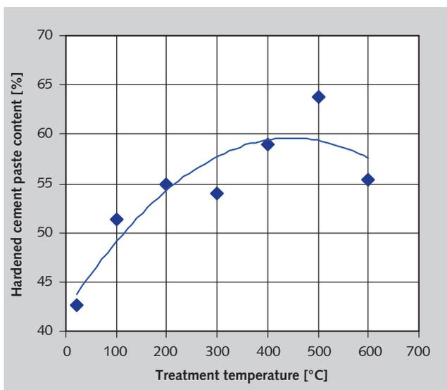
6 Influence of the temperature of the thermal treatment on the hardened cement paste content in the fine products
