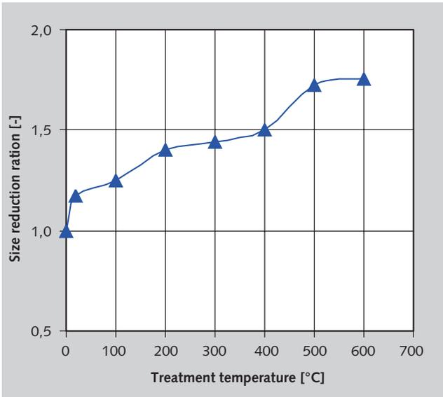
2 Starting material 8/16 mm – influence of the temperature of the thermal treatment on the size reduction ratio
