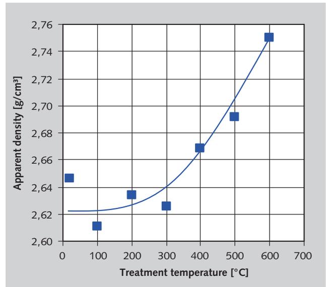
5 Influence of the temperature of the thermal treatment on the apparent density of the coarse products
