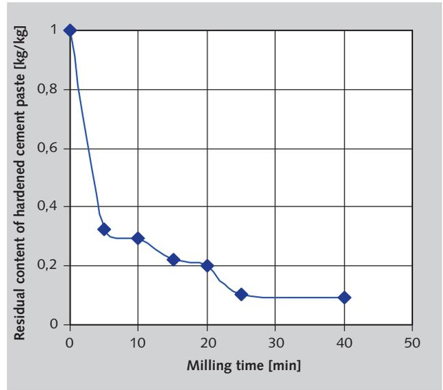
9 Influence of the milling time on the residual content of the hardened cement paste in the coarse products
