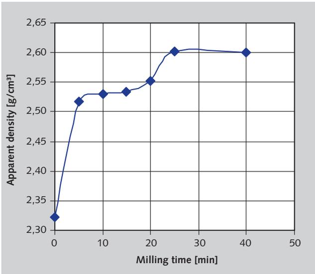
10 Influence of the milling time on the apparent density of the coarse products
