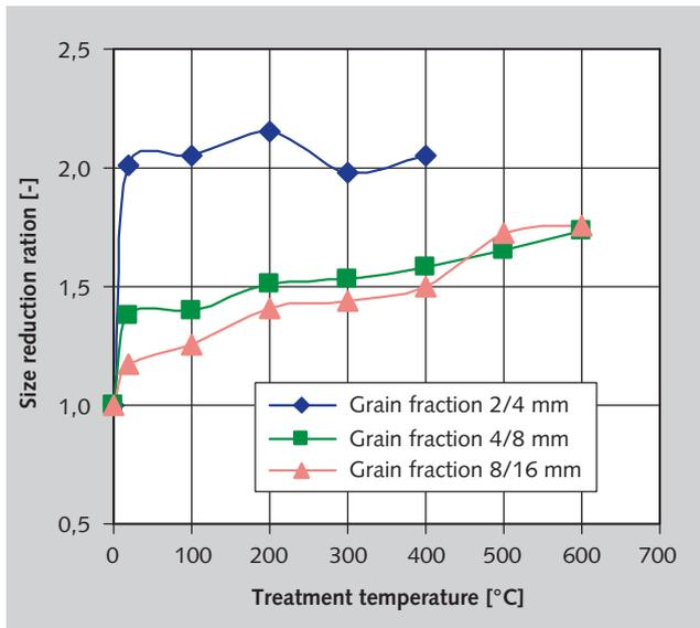
4 Influence of the particle size of the starting material on the size reduction ratio during thermal treatment
