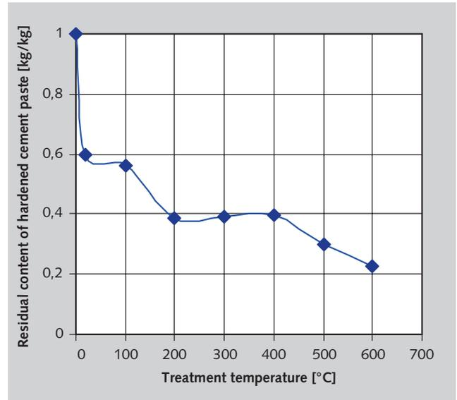
3 Starting material 8/16 mm – influence of the temperature of the thermal treatment on the residual content of hardened cement paste in the coarse product
