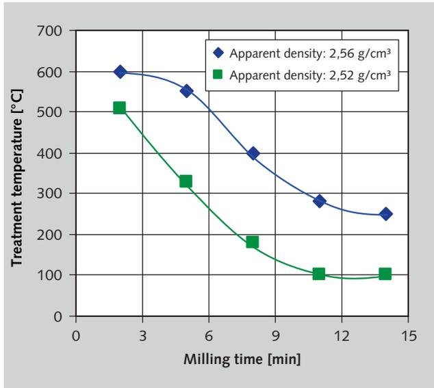
12 Starting material 4/8 – combination of the milling time and the temperature for the production of the coarse products
