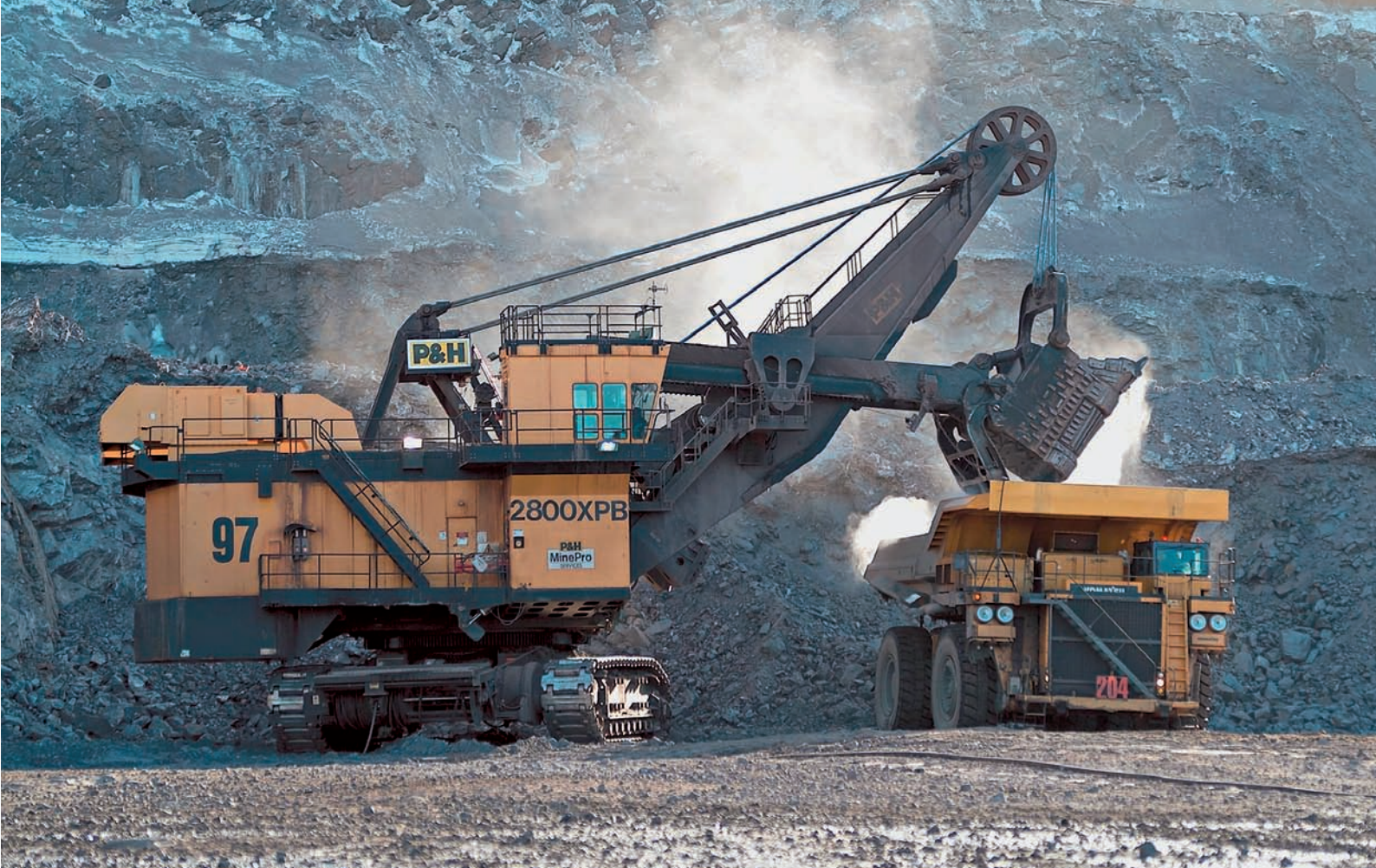
10 Truck/Shovel Methode • Truck/shovel method
